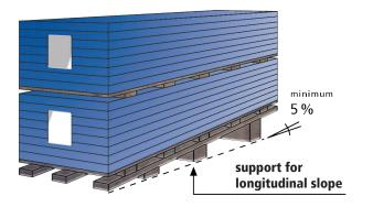
In case of storage of the packages directly on the roof, permission of the local site supervisor must be granted. Packages must be stored only on load-distributing support. Total load must not exceed the maximum load bearable by the support construction. Packages/panels are to be secured against gliding off. In case of interruption of installation work, open packages must be secured against wind exposure.
